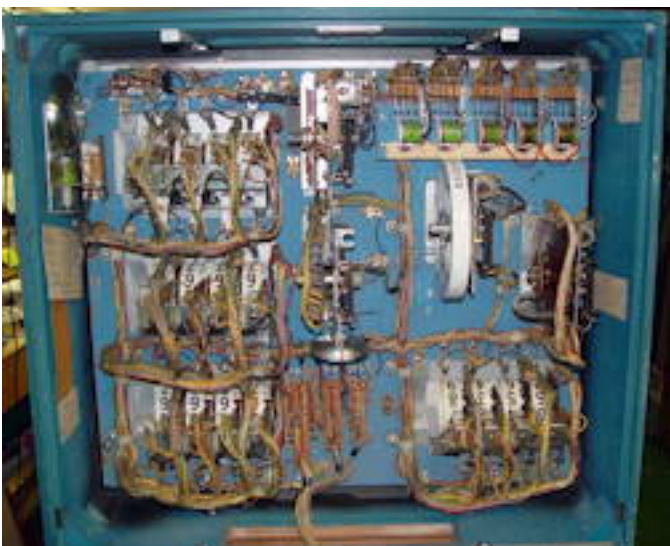
Figure 14 11 : This is the inside of the commercial EM Fireball game main cabinet. A lot of relays and stepping relays are needed because the microprocessor was still on the drawing board. Wiring this as a kit would take a lot of evenings. Not shown are the solenoids and switches on the playfield. I wonder if Bally hired engineers from the telephone company? They were the relay logic pros.
